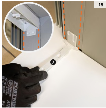
Installation with double-sided tape. Degrease and dry the fixing surface before applying the double-sided tape: full adhesion is achieved after at least 24 hours
