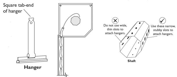
If the Rollshutter is spring loaded, the curtain should now easily roll-up with some manual assistance. It should not fly up abruptly on its own! If this happens detach the curtain hangers, then increase or decrease the pulling strength by preloading the spring more or less, it is recommended to wear protective gloves.
