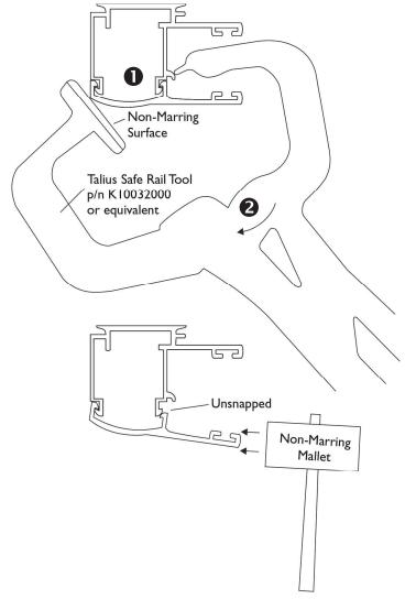
Start at the bottom of the guide rail. Using the safe rail tool, compress the safe rail mount
