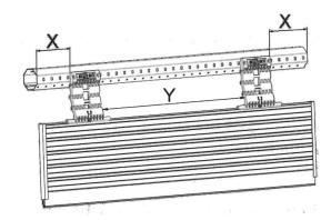
Talius supplies a special  $6-32 \times 1/4$ " screw to attach the hanger locks to the shaft. Make sure to install on the correct side of the shaft as shown below and **DO NOT** over-tighten. We recommend using a drill set to the lowest torque setting or tightening by hand.
