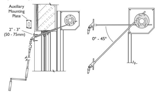
If the operator does not run through a wall the universal joint will be attached directly to the panel box in a similar manner. Most often the factory has already performed this. If the operator is mounted on a rolling door bracket frame, the connector rod is simply pushed into the gear or manual override motor and must be drilled and fastened with a cotter pin.
