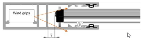
Fig. 6 - Previous version - GR100x35IE guide rail and SP/77-MSM (MSW) side lock
